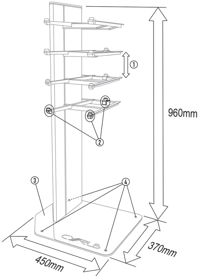
The all-metal, high rigidity HARK III framework provides a solid, stable platform (3) connected to the floor by top-adjustable spikes (4) to reduce the coupling of room vibrations into its structure.
